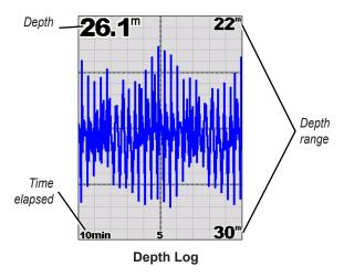
The depth appears along the right side, and the time elapsed appears along the bottom. The graph scrolls to the left as information is received
